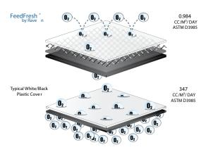
Over 350 Times Less Oxygen (O <sub>2</sub>) Passes Through FeedFresh \* Silage Covers
