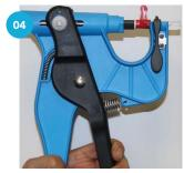
Carefully squeeze the applicator handles together, guiding the punch tip into place if necessary. When fully seated the gun bolt will rest tightly against the red plastic clip.
