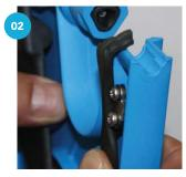
Ensure the tube retainer at the base of the applicator gun is open. Push the retainer clip to open.
