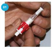
Remove a TSU Punch from the packaging. Punches should be assembled as one piece: if they have come apart, reassemble.
