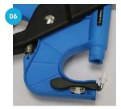
Remove the used cutter from the applicator by pulling the handles apart. This will loosen the cutter. Discard safely. CAUTION: THE CUTTER IS VERY SHARP.
