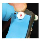
Note: The red plunger is visible in used punches.
