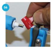
Remove the red plastic clip by pulling it outward. TAKE CARE NOT TO CUT FINGER ON THE METAL CUTTER, IT IS VERY SHARP.
