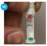
Check that sampling has been successful. If not, discard the sample and re-sample with a new punch.
